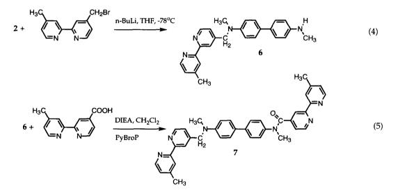
In the first step, one equivalent of n-butyl-lithium in hexane at  $-78^{\circ}$ C was added to a solution of **2**, followed by addition of one equivalent of 4-bromomethyl-4'-methyl-2,2-bipyridine. This gave ligand **6** in 46 % yield.<sup>9</sup> The product was purified on silica with precautions taken to avoid air oxidation.
