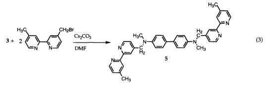
Cesium carbonate and 4-bromomethyl-4'-methyl-2,2-bipyridine were added in excess to the solution. The reaction was carried out in the dark under N<sub>2</sub>, at room temperature for 24 hours. Ligand 5 was obtained in 70% yield.<sup>8</sup> Precautions were taken in purifying and storing this ligand due to its easy air oxidation.
