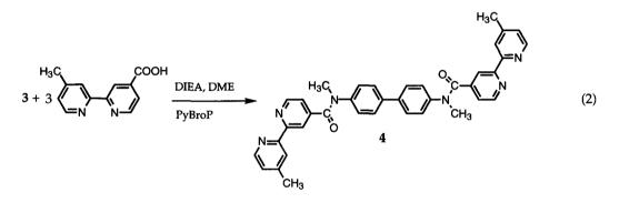
The coupling reaction was based on a literature procedure<sup>5</sup> and was conducted in the dark, under N<sub>2</sub>, at room temperature over a 12 hour period. Ligand 4 was obtained after purification on alumina with a total yield of 70%.6
